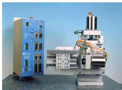
Precision x,z Stage with 25 mm travel and accuracy of 2.5 microns per half step. Optionally 1 micron per half step if 500 step motors are used. Vacuum specification > 10^{-7} mbar. Two motor Programmable Controller
