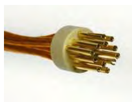
Back shell with pins during assembly
